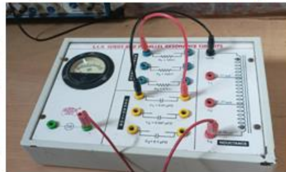
LCR Series and Parallel Resonance Circuit
