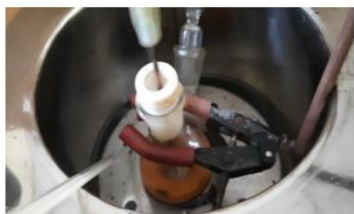
Fig.4: Experimental setup for epoxidation of fish oil.
