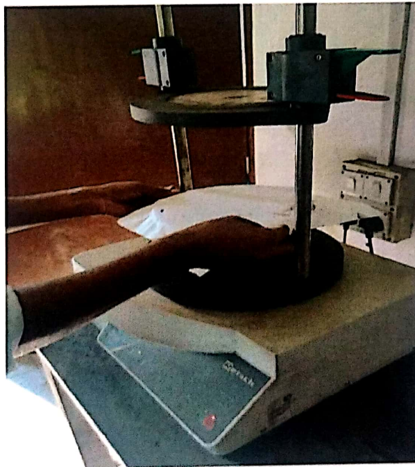
Fig 7: Crushing the sand samples in Sieve Shaker machine (212 \mu\text{m} )
