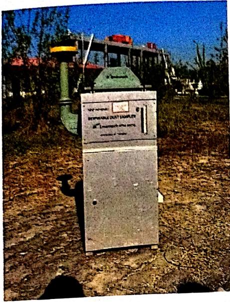
Figure5: Respirable Dust Sampler (Envirotech APM 460 NL)
