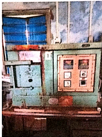
(2) Muffle Furnace (Okay Model: 60F6)
