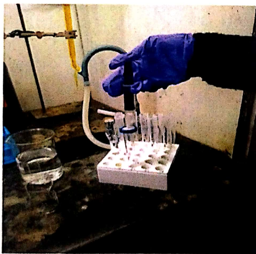
Fig 7: Digested samples diluted and filtrated using a 0.4-micron syringe filter.
