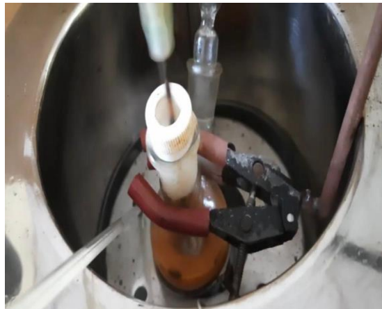
Fig. : Experimental setup for epoxidation of fish oil.
